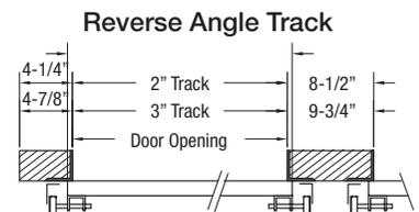
Typical Construction for Reverse Angle
